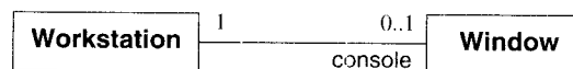
Figure 3.9 Zero-or-one multiplicity. It may be optional whether an object is involved in an association.
