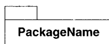
Figure 4.27 Notation for a package. Packages let you organize large models so that persons can more readily understand them.
